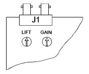
**Default Position.** For shorter cable lengths, turn the relevant control anticlockwise until the required picture quality is obtained. For longer cable lengths, turn the relevant control clockwise until the required picture clarity is obtained.
